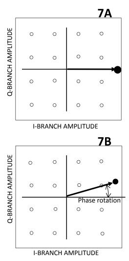
single-branch references with regular data, because none of the modulation states has zero or near-zero power in one branch, and none have zero or near-zero degrees overall phase.
