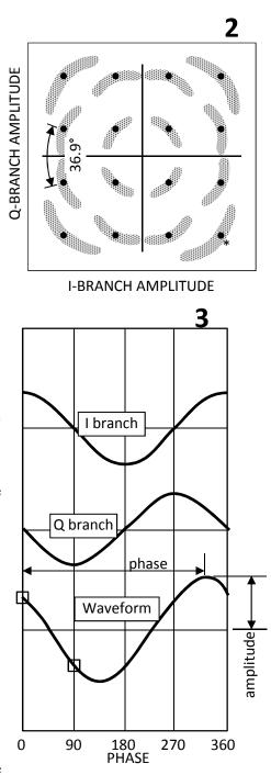
and phase from the I and Q amplitudes, or alternatively by digitizing the full waveform as it arrives. In either case, the receiver can readily determine the amplitude and phase of the as-received waveform.
